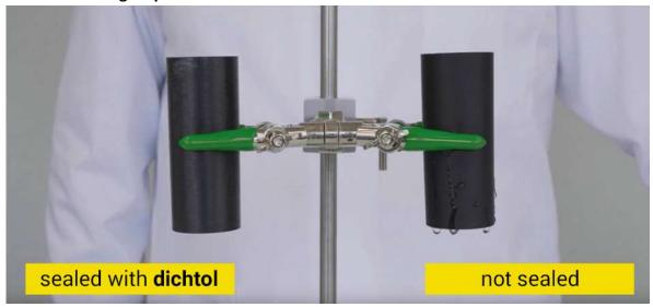
dichtol AM Hydro will penetrate deep into additively manufactured components, where it cures. Its high-performance, hard-elastic polymer delivers permanent, gap-free sealing and impregnation, preventing liquids or gases from leaking out of cylinders, vases, and other 3D printed objects.
